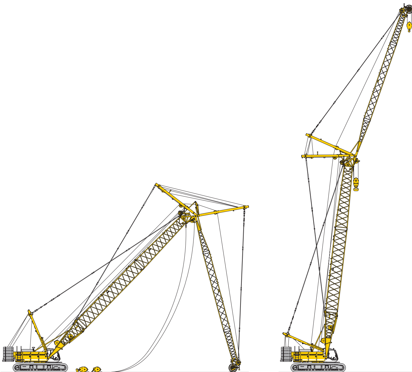
Erecting of main boom and luffing jib
