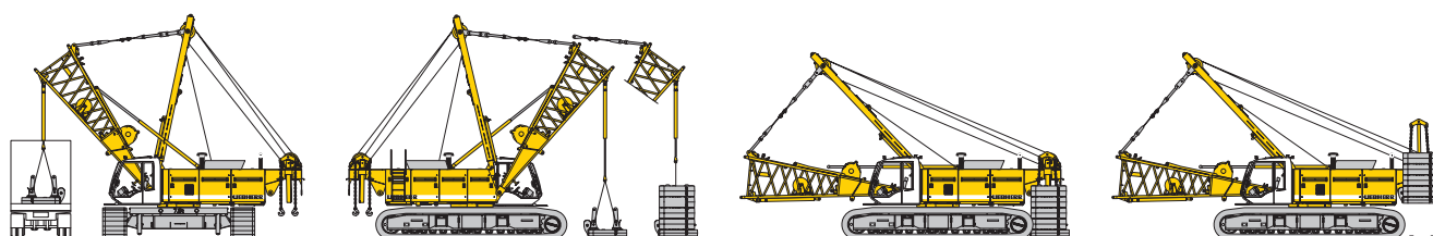
Unloading and assembly of counterweight
