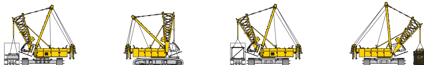
Unloading and assembly of carbody counterweight
